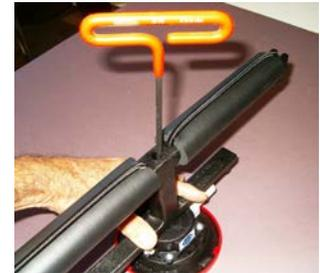
Now remove the vacuum assembly from the frame using a 3/16" hex driver placed through the top center of the rod transport frame.
