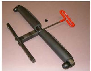
Using the 1/4-20 Finish Hex Nut provided, re-secure the frame assembly.
