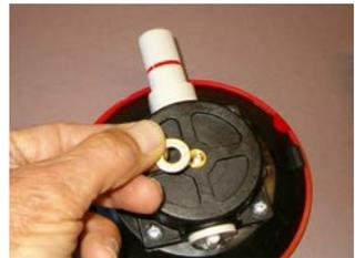
Next remove the 1/4" washer found between the frame bottom and the vacuum assembly.
