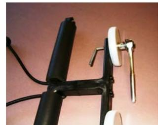
Install the Magnets using the 1/4-20x7/8" button-head bolts and the 1/4-20 KEPS Locknuts provided. This requires a 7/16" socket and a 5/32" hex wrench.
